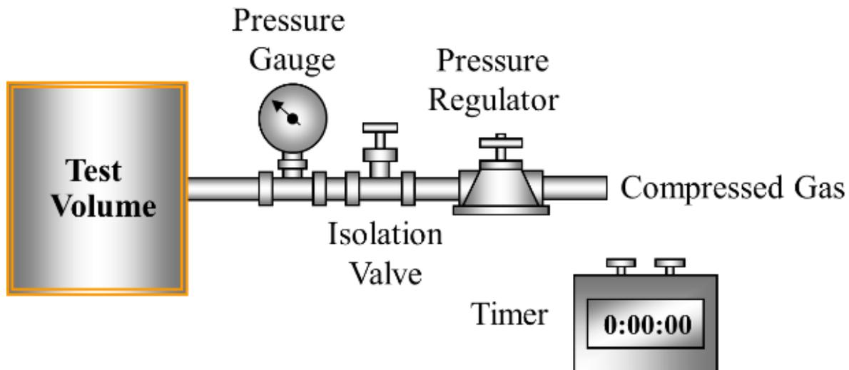
Air is simply injected into a test object, after which the pressure source is valved off. Any decrease in air pressure over time signifies a leak.
