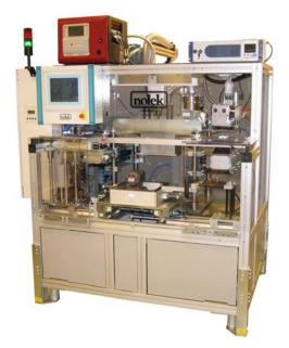
Measuring method: Helium based or Pressure decay
