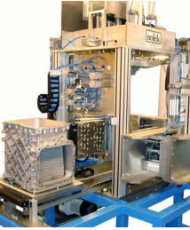
Measuring method: Pressure decay Leak rate range: 10<sup>-1</sup>cm<sup>3</sup>/sec to 10<sup>-4</sup>cm<sup>3</sup>/sec Cycle times: from 8 seconds and up Automatic calibration Compact design Available with single or double tooling
